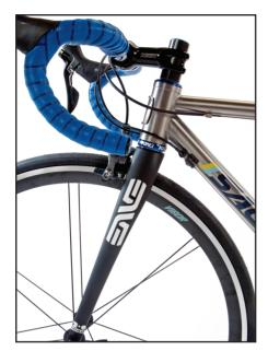
Our test bike came with a carbon Enve 2.0 fork which, combined with the 44mm head tube, provided enough front-end stiffness to give the bike a solid steering feel.
