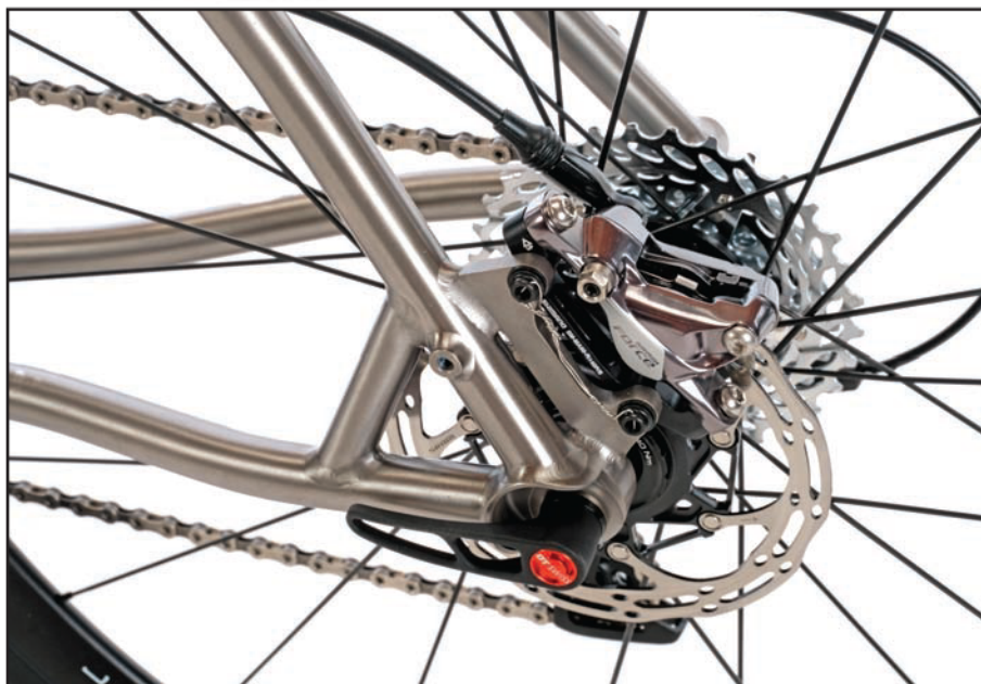
Added triangulation helps diminish any brake-induced flex.
