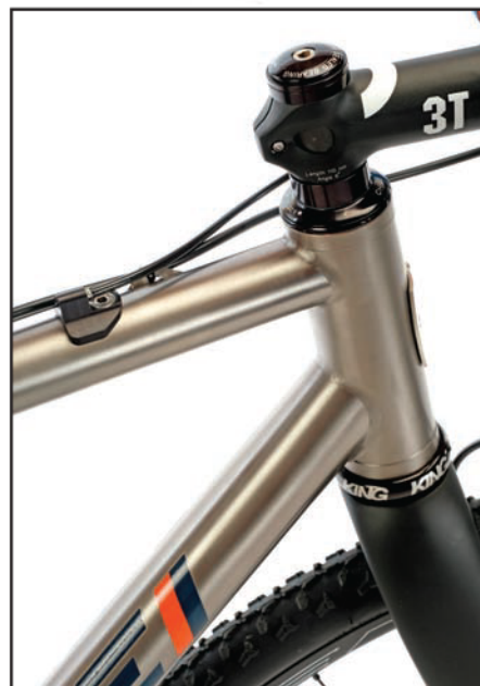
Top tube cable routing is key for cyclocross.
