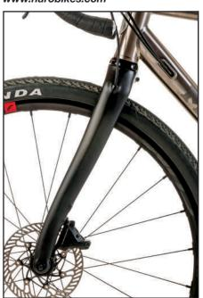
Masi's shapely proprietary carbon fork gives the Incanto's slack front end an eyecatching flair.
