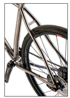
Titanium craftsmanship is put on display by the Storm King's shapely seatstays. They allow clearance for up to 700x50 tires.
