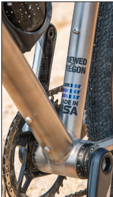
The T47 bottom bracket is a welcomed touch for the made-in-the-USA titanium gravel frame.
