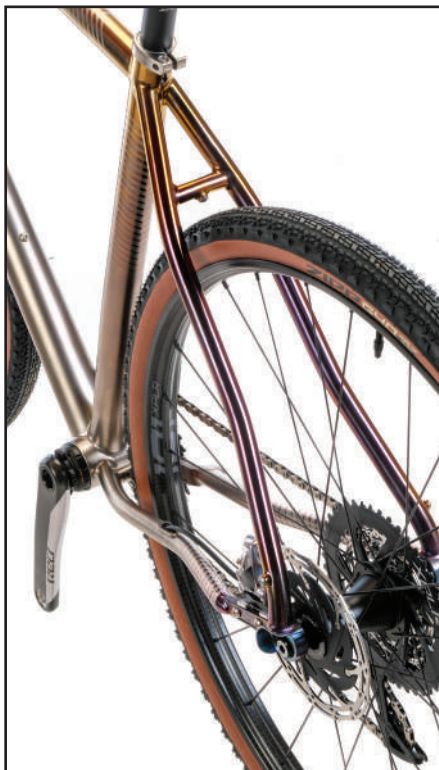
The sculpted seat stays and chainstays leave room for large 50mm tires, as well as fenders.
